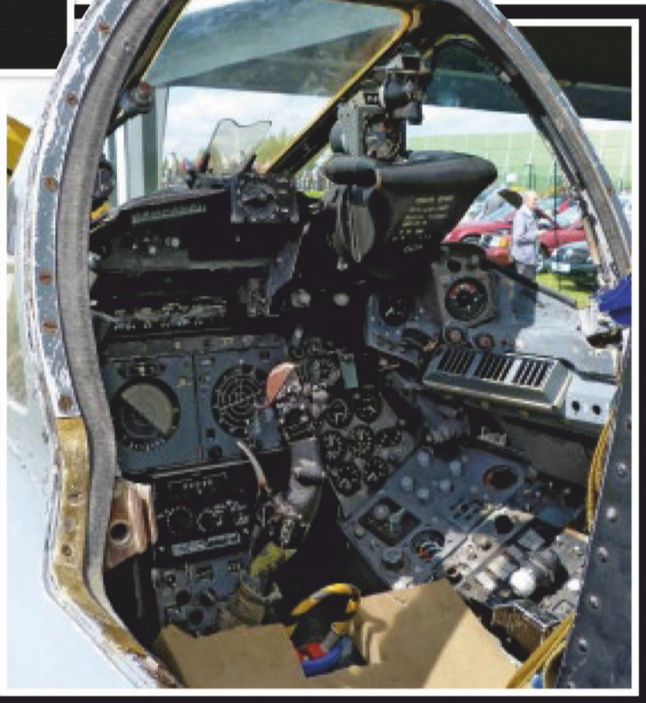
Below: The linear 'strip' speed display that replaced the conventional dial in the F.6
